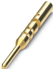
Crimp contact, turned, contact diameter: 0.8 mm, crimp range: 0.08 mm<sup>2</sup> ... 0.25 mm<sup>2</sup>
